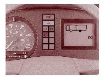
Alternatively, in vehicles without such a display, errors can also be reported via a red and a yellow warning light. A separate TCS light then indicates to the driver the ongoing TCS control activities.
