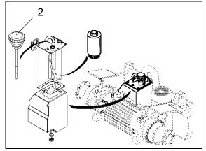
Visually check hydraulic oil level at dipstick (3).
