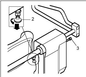
In the event of a power failure, the support system can be unlocked by means of pulling knob (3). The safety straps can then be swivelled backwards manually.
