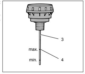
If required, refill hydraulic oil up to the required level (10 mm at dipstick (3) correspond to approximately 1 l hydraulic oil).
