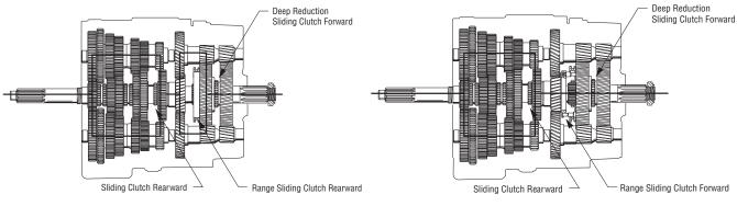
Figure 2-7. Reverse Gear-Low Range
