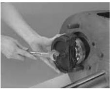
8. Use the appropriate bearing puller T9 or prybars to remove the countershaft front bearings.
