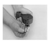
2. Install the relief valve spring in oil pump housing.
