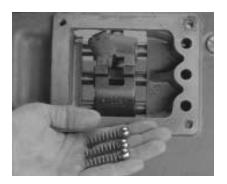
9. If the three (3) sets of tension springs and balls from the housing top bores are loose, tilt the assembly and remove them.
