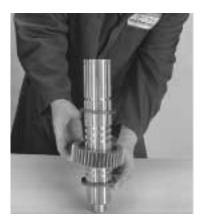
4. Remove the offset washer and 1st gear.
