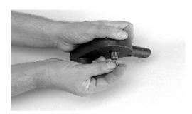
4. From the drive shaft keyway, remove the key.
