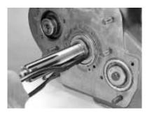
2. If present, remove and discard the rubber seal ring on the input shaft. The ring is used only to seal the transmission during shipment.
