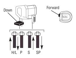
1. A tee fitting on the low range port of the slave valve will supply air through a 5/32" or 1/8" air line to the "H/L" port on the shift knob. Because this line is connected to the low range port, air is only available when low range has been selected.
