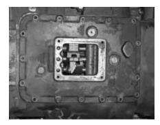
3. On the shift bar housing top, install the washer and nut.
