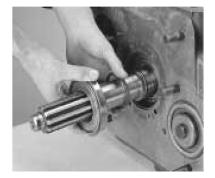
7. Remove the drive gear internal snap ring.
