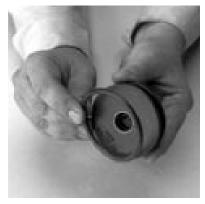
4. Install gasket and shift cylinder.
