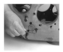
4. Remove three (3) allen head capscrews and washers that retain the integral oil pump to the case. 5. Remove the integral oil pump assembly from inside the case.
