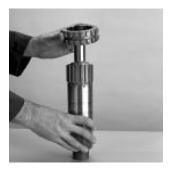
2. Mark, with toolmaker's dye, two opposing teeth on the low range gear.
