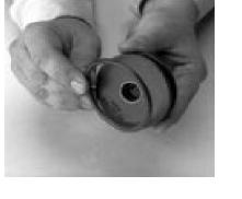
4. Install gasket and shift cylinder.
