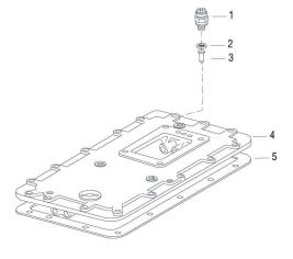
1. Reverse Light Switch 2. Gasket 3. Pin 4. Shift Bar Housing 5. Gasket
