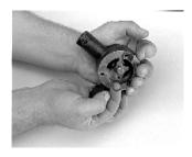
9. Install the inner element retention snap ring in drive shaft snap ring groove.
