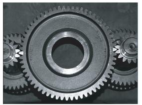
Example showing correct view of Reduction gear timed to Countershaft gears on the bench.
