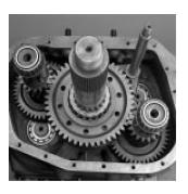
11. Assemble mainshaft assembly into transmission rear. Splines on mainshaft end must slide into range synchronizer. Marked teeth on low a range gear must be aligned with marked teeth on countershafts.
