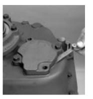
8. Average the two feeler gauge measurements by adding the measurements together and dividing by 2 as shown in Example.
