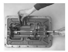
4. While removing the top yoke bar to the right, remove the two (2) shift blocks.
