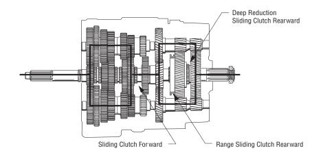
Figure 2-4. Front Section Power Flow
