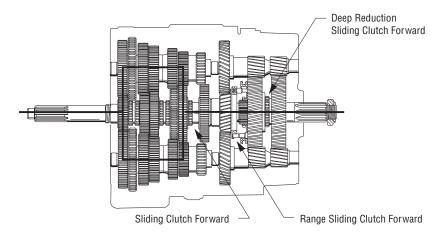
Figure 2-10. High Range Selected (Range Sliding Clutch Forward)
