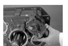
5. Install range piston with flat side to rear. Install range piston nut and torque to 70-85 Lb•ft.
