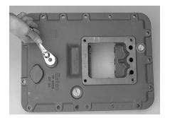
3. On the shift bar housing top, install the washer and nut.
