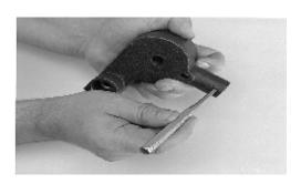
10. From the pump housing, remove the relief valve roll pin.
