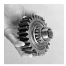
5. Inspect the reverse gear assembly, remove the inner race and needle bearing, if damaged.
