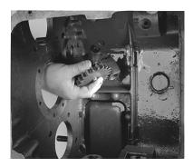
4. Align oil pump with retainer and alignment pin and install the integral oil pump assembly.
