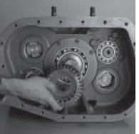
2. Slide the auxiliary drive gear off the mainshaft.
