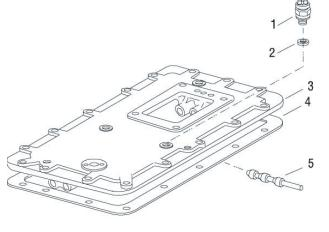
1. Neutral Light Switch 2. Gasket 3. Shift Bar Housing 4. Gasket 5. Air Valve Shaft
