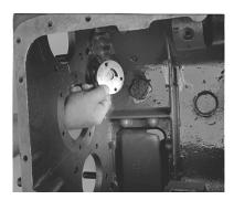
3. With the retainer bore facing the case rear, install the integral oil pump over the alignment pin inside the case.
