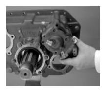
8. Install gasket and cover. Apply Eaton® Fuller® thread sealant P/N 71205 or equivalent to capscrew threads. Install capscrews and torque to 35-45 Lb•ft.
