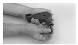
11. From the relief valve housing bore, remove the relief valve spring.
