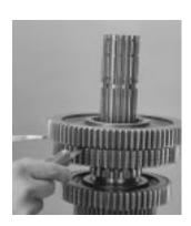
15. With clutching teeth down, position the next gear on the mainshaft engaging with spacer external splines.
