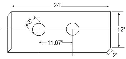
This fixture is designed to ease the assembly of the auxiliary gearing. Set the auxiliary countershaft rear bearings in the 3" holes.
