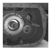
3. Move the countershaft to the rear and insert the countershaft support tool to center shaft in rear case bore.
