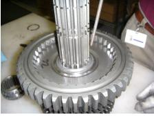
15. With clutching teeth up, install the 1st gear on the shaft against previously installed gear.
