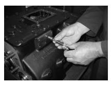
6. Install interlock parts (pin, spring and sleeve).
