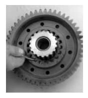
3. Assemble low range gear to coupler and install bushings if removed.
