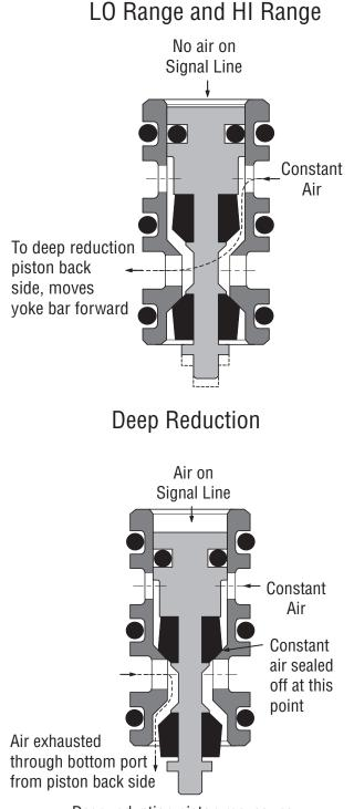
Deep reduction piston moves rearward due to constant air on front side.
