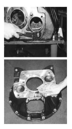
5. Remove the gasket and clean all mounting surfaces of gasket material.
