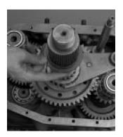
14. Install stepped washer over auxiliary mainshaft with stepped side up.
