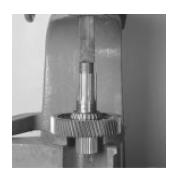
10. Remove the bearing inner spacer from the output shaft.
