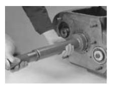
5. Install the input shaft bearing over the input shaft. Use a flanged-end bearing driver which contacts both the bearing inner race and outer race. Drive the bearing until it contacts the front case.
