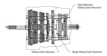
Figure 2-6. Reverse Gear-Deep Reduction
