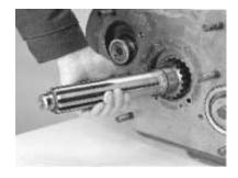
4. Use a soft bar and maul to drive the input shaft toward the case rear as far as possible. Pull the input shaft forward.
