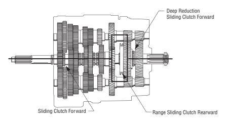
Figure 2-5. Front Section Power Flow - Direct Gear
