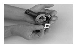
7. From the drive shaft keyways, remove the two (2) keys.
