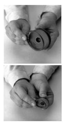
7. Remove the cylinder housing and gasket.
