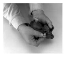
5. Install range piston with flat side to rear. Install range piston nut and torque to 70-85 Lb•ft.
