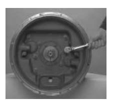
4. Pull the clutch housing from the studs and transmission case.
