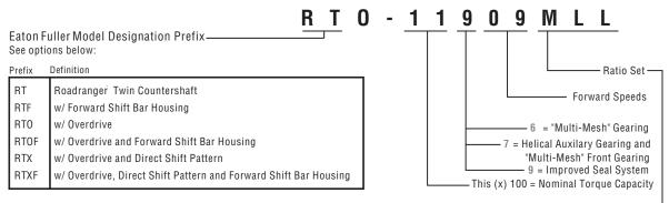
L or LL notation used here indicates one (L) or two Low (LL) gears in addition to designated speeds  $\_$
