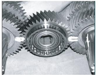
7. To ensure the timing is correct, check that the marked tooth on the Splitter gear is between the two marked teeth on the Auxiliary Countershaft gears as shown in the illustrations below.
