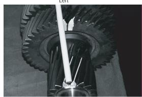
4. Use a round file or bar to properly align from the marked teeth on the Auxiliary Countershaft to the Auxiliary Splitter gear. When the bar is lined up with the root, between the correct teeth, you will notice it's parallel with the Auxiliary Countershaft. Mark both the teeth with a highly visible paint.
