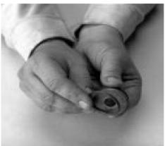
7. Remove the cylinder housing and gasket.
