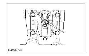
12) Move the bearing cap with hand, and release and reassemble it if no movement is detected.
