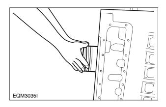
Remove the piston pin snap rings, take off the piston pin, then disconnect the conn. rod from the piston.
