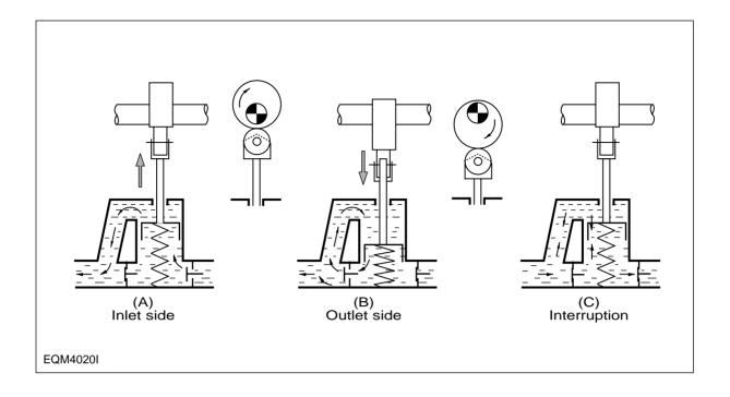
This feed pump is mounted with a priming pump designed to permit manual feeding of fuel from the fuel tank with the injection pump mounted in the engine. During the manual feeding operation, air must be bled from the fuel lines.
