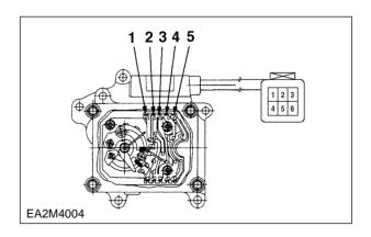
(3) Check the resistances between each of the rack sensor terminals shown in the figure using a circuit tester. Their resistances at 25°C are shown in the table below.
