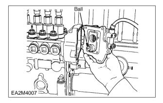
(2) Confirm that the actuator's pre-stroke position sensor plate moves smoothly when moved with a finger, as shown at left.
