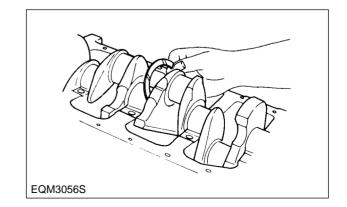
Install the bearing and thrust washers to the bearing cap and apply oil to the bearing and thrust washers.
