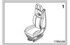
The belt does not need to be adjusted by hand: the webbing adjusts itself automatically to the length most suited to the driver allowing him freedom of movement provided that his movements are not abrupt. The belt mechanism is affected by changes in vehicle attitude and as a consequence the belt may lock in the following cases:
