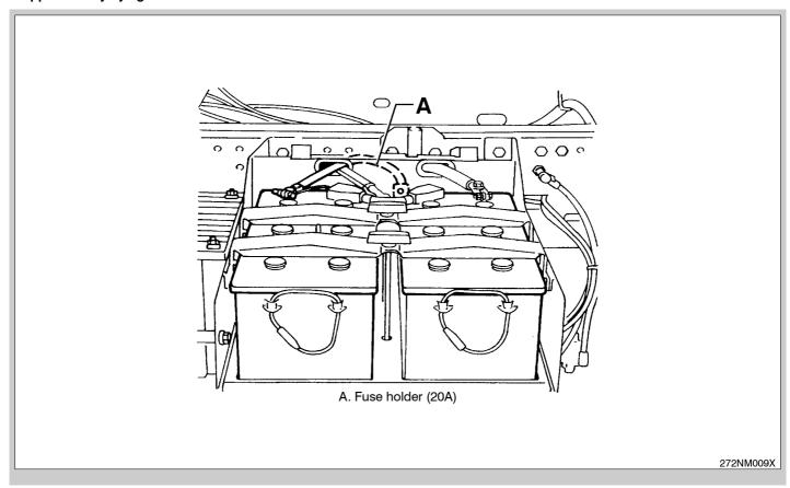
There is a flying fuse holder near to the batteries, which contains a 20A fuse.
