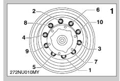
unlock the fastening nuts completely and remove them, then withdraw the wheel, taking care not to damage the stud bolt threads;
