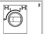
Reat longitudinal distributor and transverse differential lock (4x4 vehicles only) (Fig. 2)
